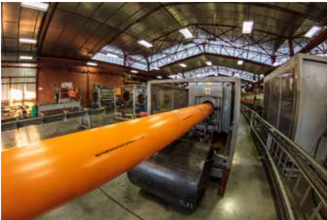
FIGURE 3.12A: EXTRUSION OF AN HDPE GAS PIPE
