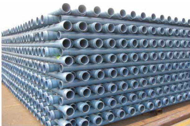
FIGURE 6.1: STACKING OF PVC PIPES
