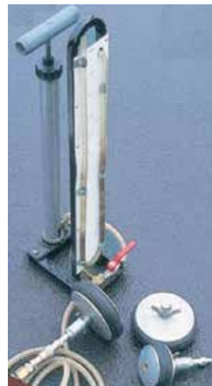
FIGURE 4.23: AIR TESTING EQUIPMENT
